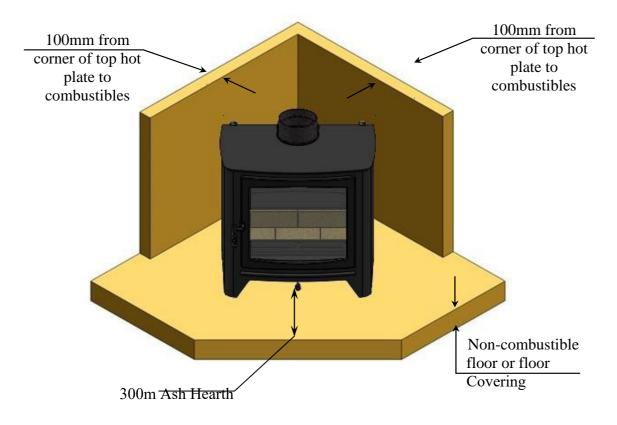
These clearances can be reduced by using shield as stated in ASNZ 2918 Note: combustible material refers to any material that will degrade when subjected to heat e.g. plasterboard
